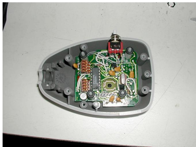
This photo shows the front half of the case with the board and switch installed.
