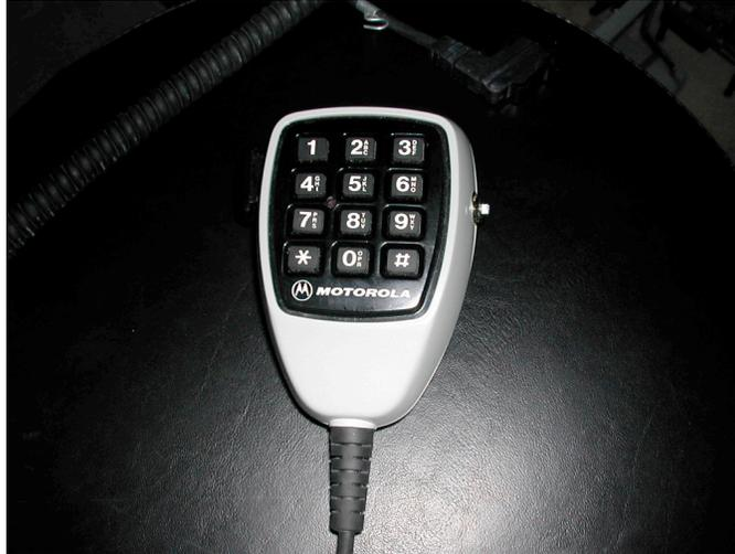
This photo shows the finished microphone. I took a small pair of diagonal cutters and trimmed the handle on the switch so that only enough protrudes to make it easy to activate.
