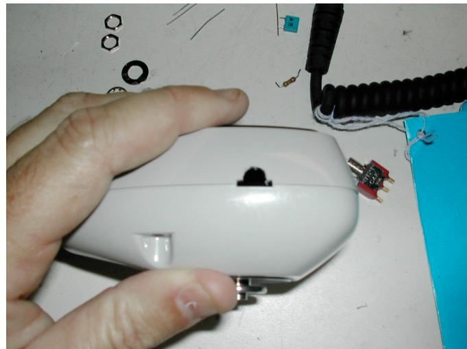
Next, plug the keypad back into the DTMF generator board and install the board, with switch, back into the front half of the microphone case.
